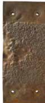
Used apron plate with minimal wear after 74,000 tons
